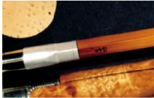
The transition from ferrule to blank is wrapped as well.
