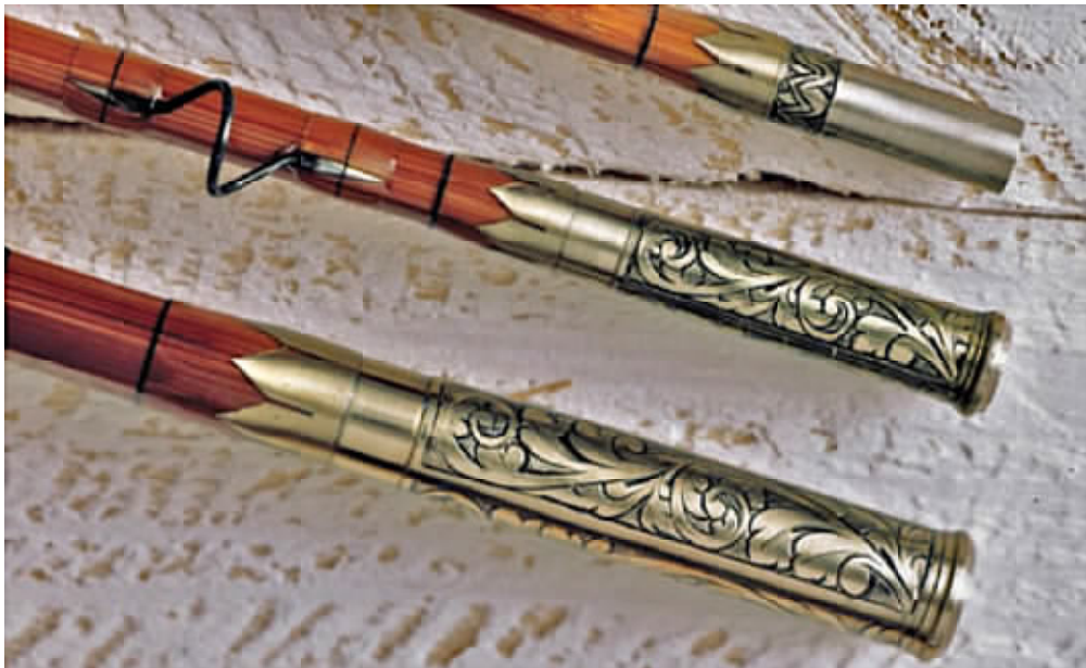
When a finish is applied, white silk loses its color and becomes transparent.
